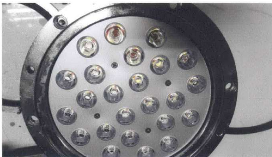
Photo 4: Test result after IP6X and IPX8 test
