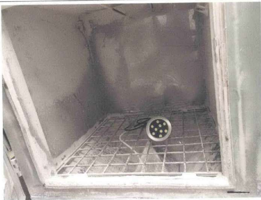
Photo 3: IP6X test of model 61063
