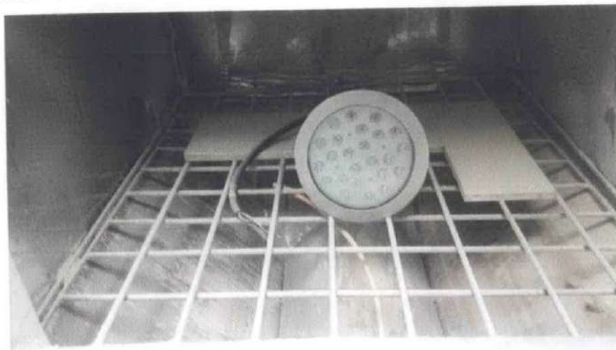
Photo 2: IP6X test of model RS-UW96W316X
